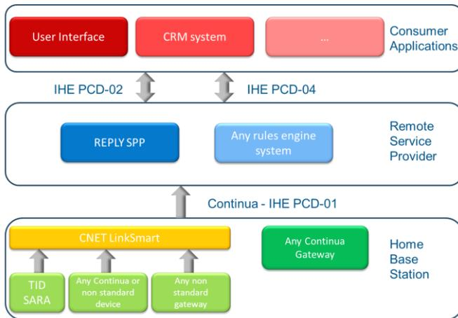
**Figure 5 Interoperability of the inCASA architecture**
