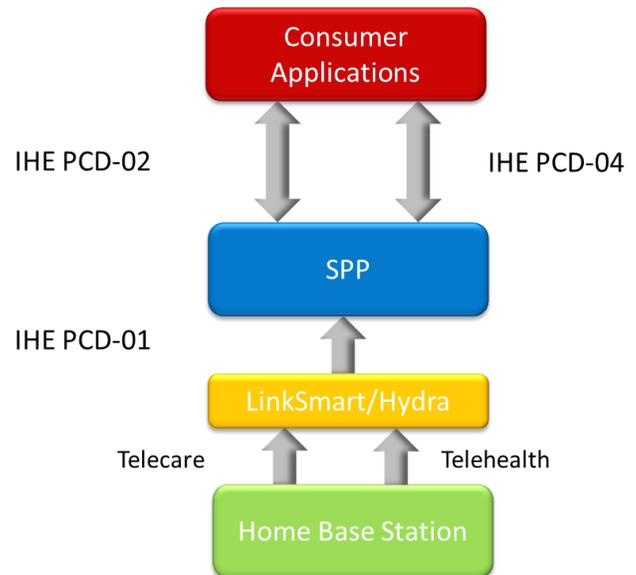
**Figure 4 Integration between the inCASA platform components**
