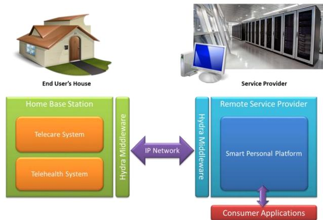
**Figure 3 Technological architecture of the inCASA platform**
