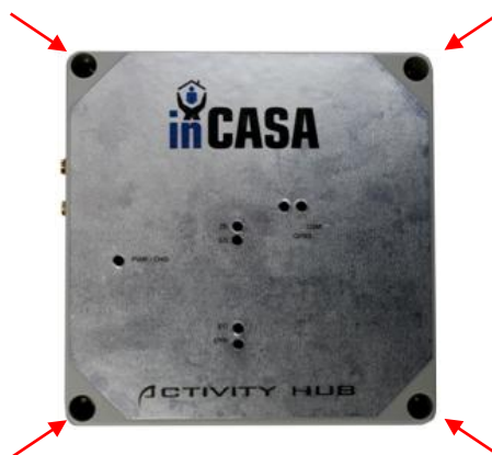
Figure 3: Opening the AH by removing the screws
