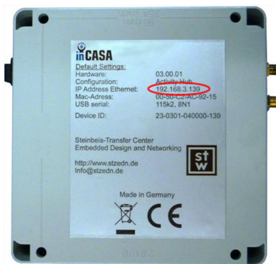
Figure 12: AH identification plate with factory default IP address
