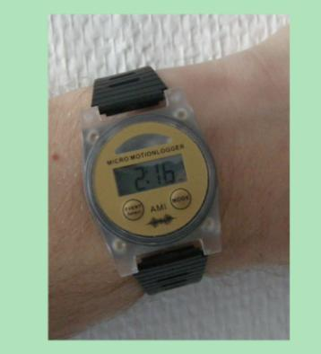
dongle. This Actigraph, developed by Ambulatory Monitoring Inc. (Ardsley, NY, US), is a new version which includes infrared communication for data transmission. Patients are asked to wear the device as a watch day and night and to download the data to the electronic platform once a day using the infrared dongle. The sensor measures the number of accelerations per minute in order to assess the rest-activity rhythm. The downloaded files are sent to a server to be analyzed by the pilot team.
